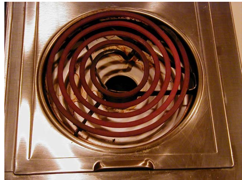
Visible-light picture of a stove element (Temperature ~ 400 K)
