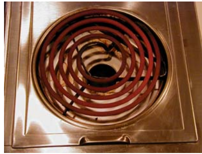
Visible-light picture of a stove element (Temperature ~ 400 K)
